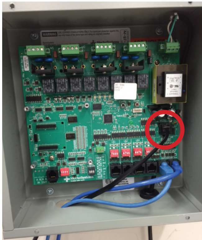
Figure 2. RS232 inside the MechoSystems IQ/MCL2 Controller
