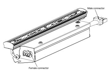
2. Prepare beginning fixture for line voltage input by removing top screws to open wiring compartment. Remove male connector wiring from fixture and discard. Feed power lead cable (by others) through right side hole and trim to desired length. Connect power lead cable and input driver wiring to female connector wires via wire nuts. NOTE: Minimum of 18 AWG power lead cable wires to be
