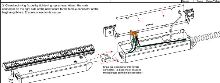
4. Continue to connect each additional fixture in the series using the connectors. Do not exceed the maximum allowable run length (See table above).
