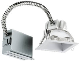
Junction Box Fixture Kit with 4" Square Reflector Ceiling Cutout: 5.00" Retrofit / 5.125" New HCD 4-inch Square spec sheet
