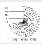
HLBT609FS5\*-930 Spacing criterion: (0-180) 1.26 | (90-270) 1.26 | (Diagonal) 1.38 Beam Angle: 111° Field Angle: 160° Lumens: 965 Input Watts: 9.7 W Efficacy: 99.5 LPW UGR: 26.8 Test Report: P832732
