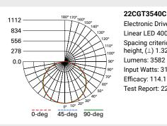
Electronic Driver Linear LED 4000K Spacing criterion: (II) 1.32 x mounting height, ( $\perp$ ) 1.32 x mounting height Lumens: 3582 Input Watts: 31.4W Efficacy: 114.1 LPW Test Report: 22CGT3540C.IES
