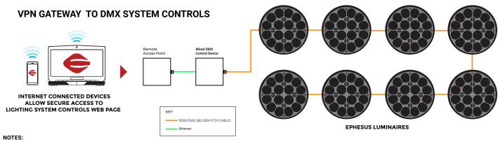
Remote Access Point requires either a wired internet connection at the lighting system site or through a cellular carrier network connection plan
