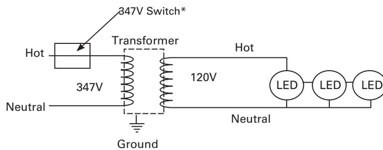
\*Use of a dimmer ahead of the transformer is not recommended
