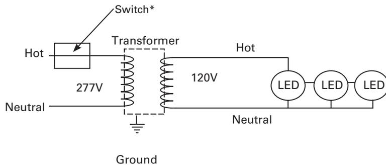
\*Use of a dimmer ahead of the transformer is not recommended
