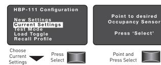
Current Settings allow you to recall the parameters for a specific sensor. These are read only parameters.
