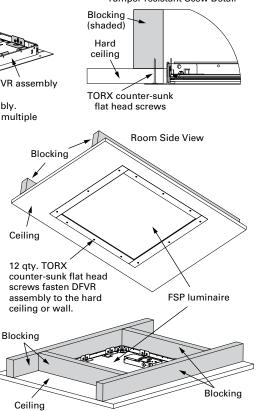
Position the DFVR assembly in the ceiling cut-out, and secure with multiple tamper-resistant screws; shown above.
