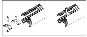
Secure end caps to the fixture using the provided **#8-18 x** ½ **HWH screws(C)**. The decorative end plates can then be mounted to the pre-installed magnets on the center of the end cap.
