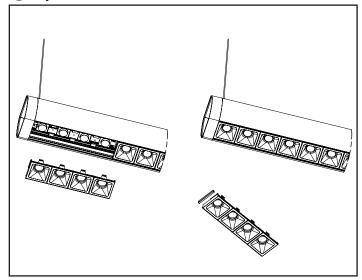
If required, use provided gaskets to ensure there is no light leak between each baffle section. (The bottom color of the gasket should match the color of the baffle). The baffles snap in and out of the fixture.
