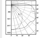
8VT2-LD5-16-DR-W-UNV-L840-CD2-WL-U **Electronic Driver** Linear LED 4000K Spacing criterion: (II) 1.22 x mounting height,  $(\perp)$  1.59 x mounting height Lumens: 15236 Input Watts: 117W Efficacy: 130.2 lm/W Test Report: 8VT2-LD5-16-DR-W-UNV-L840-CD2-WL-U.IES
