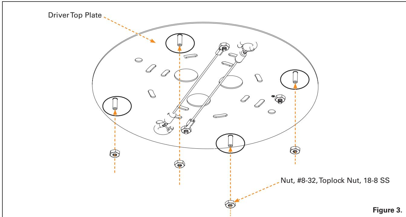
**Step 1.** Preload the Top lock nut to the Driver top plate. Figure 3
