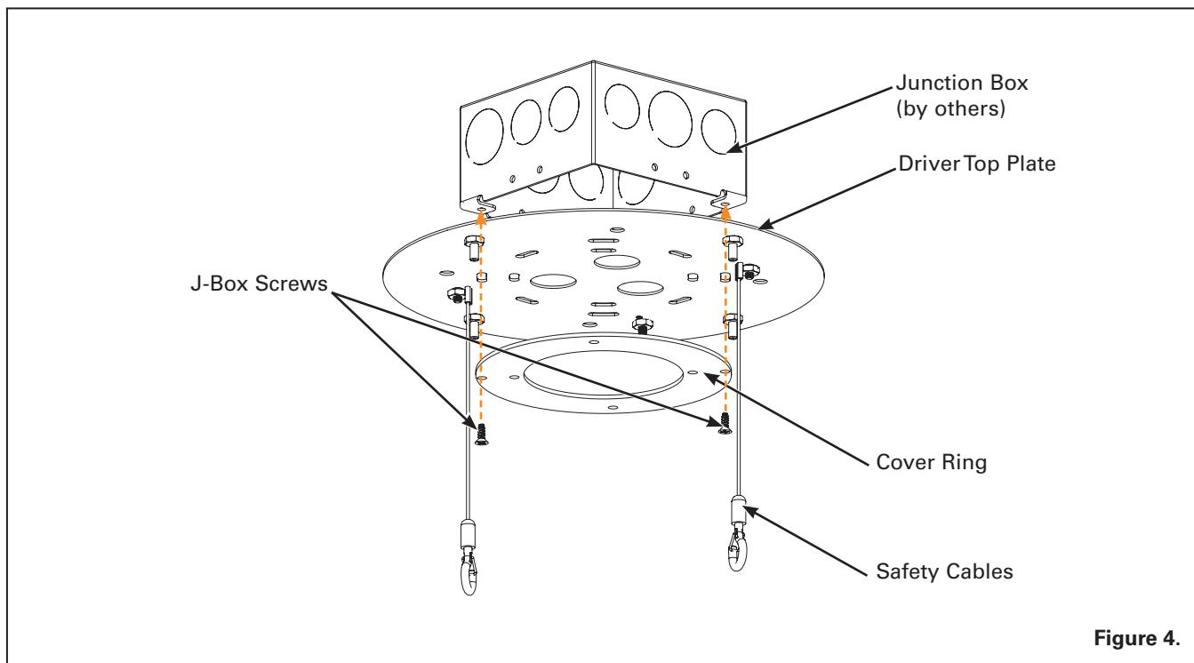
**Step 2.** Using the J-Box screws, align the Cover Ring to inside of the Driver Top Cover. Screw the cover ring and the driver top plates to the J-Box. The Cover Ring must be used to reinforce the center of the Top Plate. Figure 4
