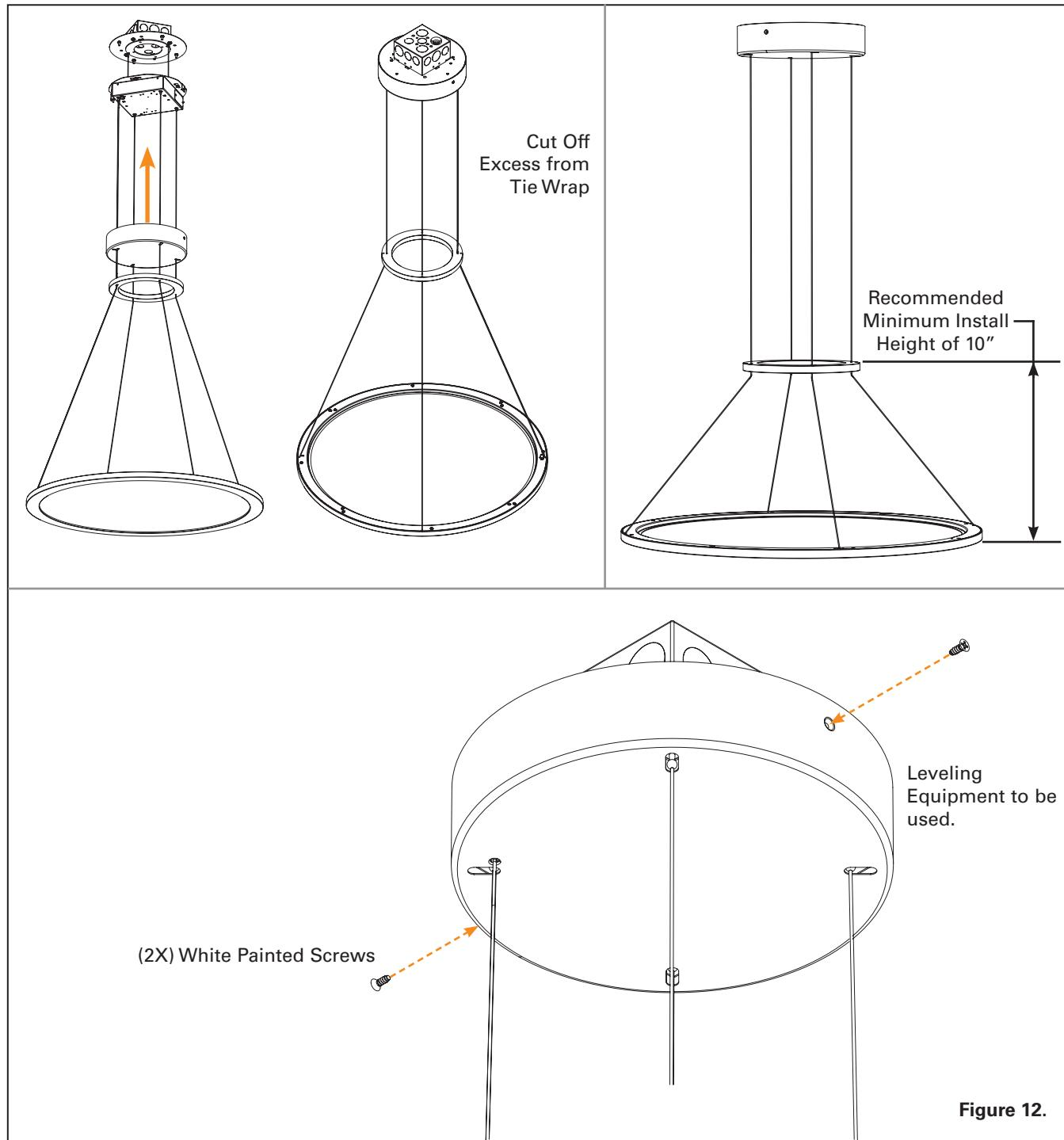
**Step 13.** Raise Decorative Cover and attach to the Driver Compartment using 2X M4 flat head screw (head painted white). Use Tie Wraps to keep the Low Voltage Cable taut against the Air Craft Cable. Ensure all wires are inside driver enclosure and ensure no pinched wires. Figure 12
